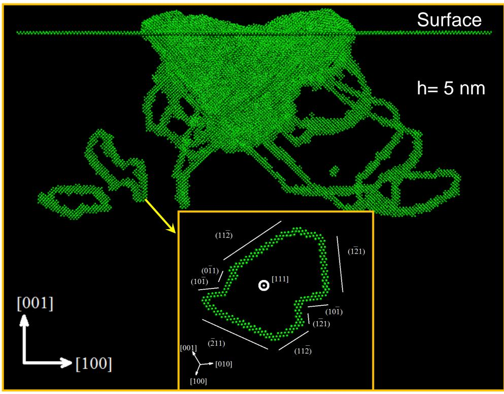
5 nm penetration image of non bcc atoms for a simulation using Ravelo's EAM potential [4]. Prismatic loops are already visible being formed by virtue of the interaction of {110} and {112} slip systems. For the highlighted loop, all the planes share the same [111] direction.
